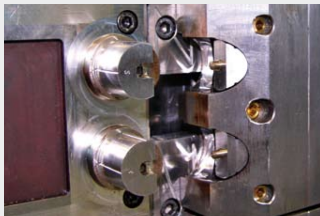
Mould contour on the ejector side with slider mechanism. The dosing pins are exchangeable.
