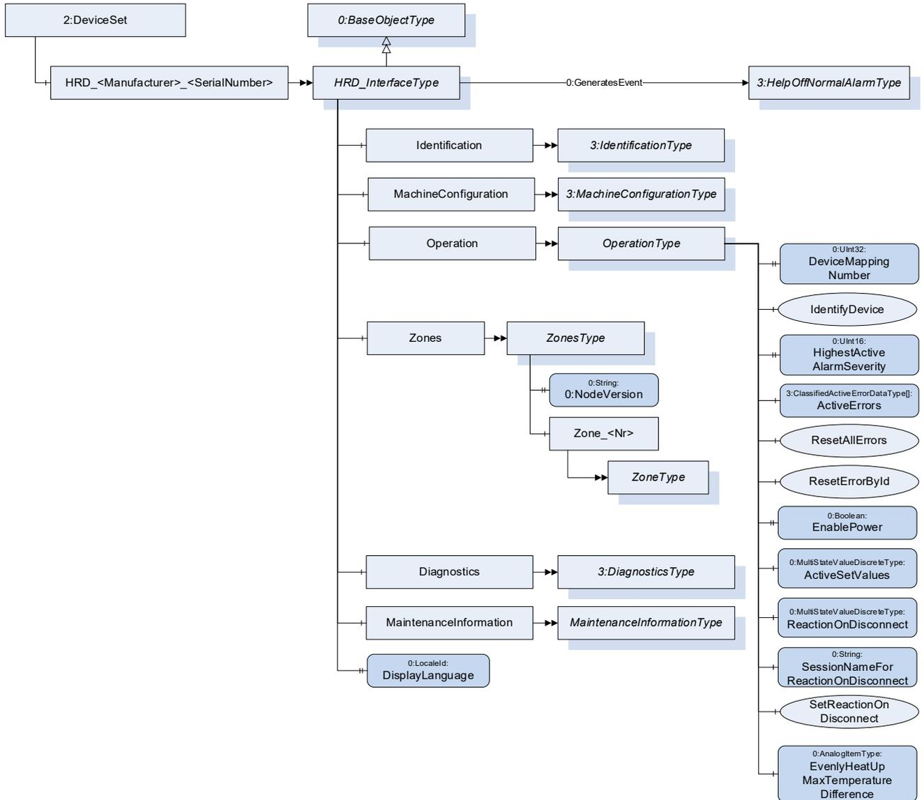
The schematic above represents the information model defined by OPC 40082-2. The pro CONTROL OPC UA server strictly follows that specification and presents the node model under DeviceSet.HRD\_EWIKON\_<SerialNumber>
