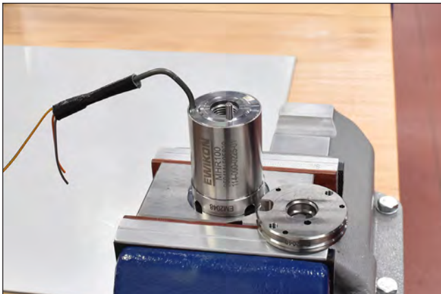
Picture 119: Disassemble the retainer ring
