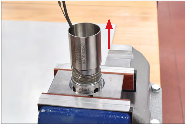
Picture 120: Disassemble the protective tube
