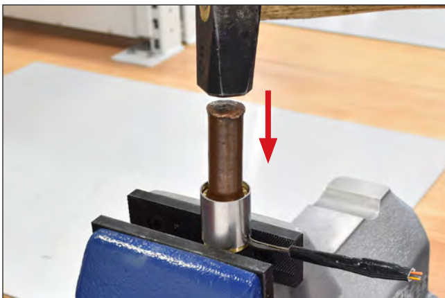
Picture 101: Disassemble the protective tube
