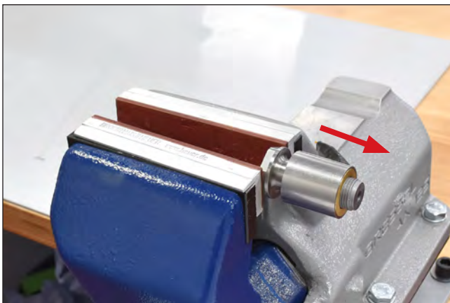
Picture 100: Pull off the heating element from the adapter
