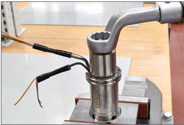
Picture 118: Clamp the nozzle, disassemble the adapter
