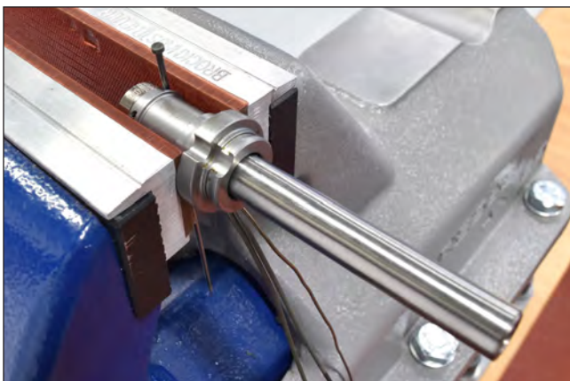
Picture 82: Pre-centre before installing the spring pins
