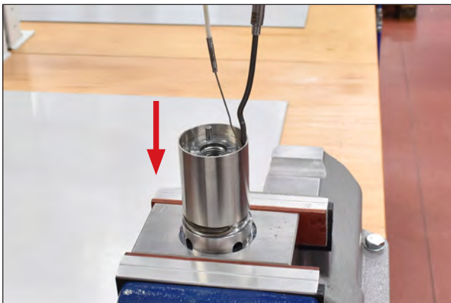
Picture 122: Installation of the new thermocouple, installation of the protective tube
