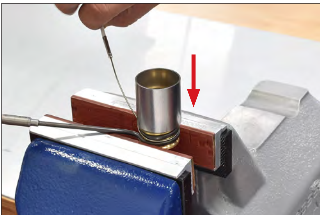
Picture 105: Installation of the protective tube
